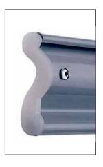
Guide made of 1,5 - 2mm thick, "Ω" shaped galvanized steel that works together with a special aluminum profile and brush strip to reduce friction and noise.
