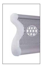
Guide made of 1,5 - 2mm thick, "Ω" shaped galvanized steel that works together with a special aluminum profile and brush strip to reduce friction and noise.
